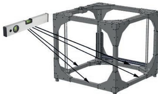
Fig. 4-4: Alignment of the frame with spirit level
